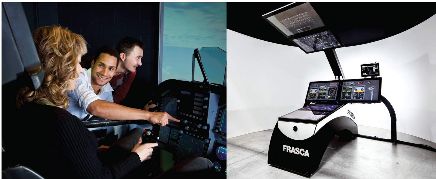
Figure 9-4. A level 4 FTD used for procedure training.
